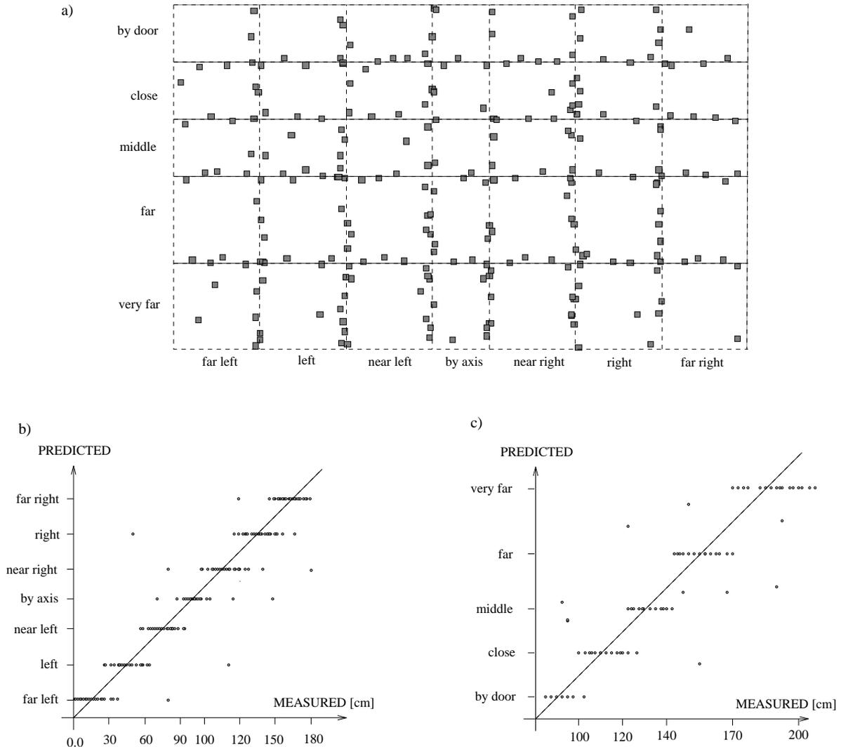
Figure 5. Distribution of prediction errors over door's neighbourhood: a) incorrect predictions (filled squares) are placed most often along the border lines of the topological clusters; b) and c) correspondence of real locations and predictions generated by the trained system for x and y axes of the door's coordinates.
