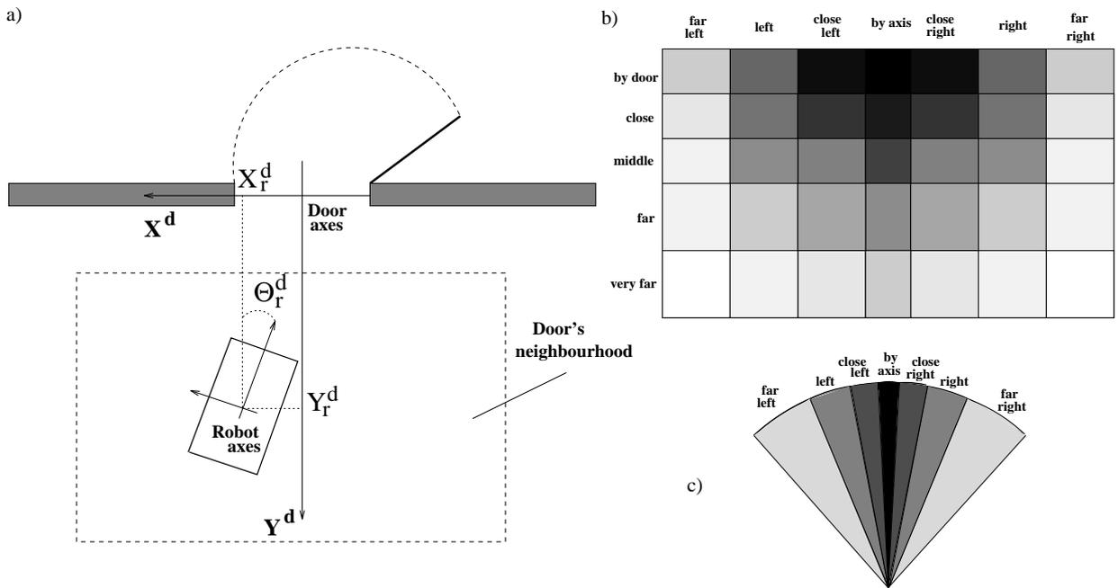
Figure 3. Robot in front of the door: a) metric description; b) topological categorization of the position coordinates; c) topological categorization of the orientation angle.
