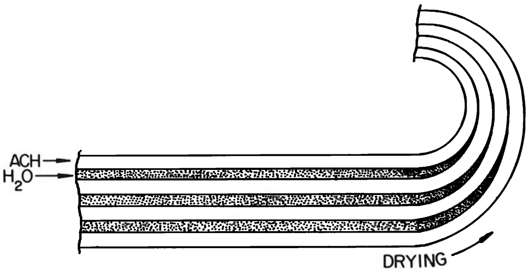
Figure 3. Schematic effect of drying on material composed of alternating layers of aluminum chlorohydrate (ACH) and water.
