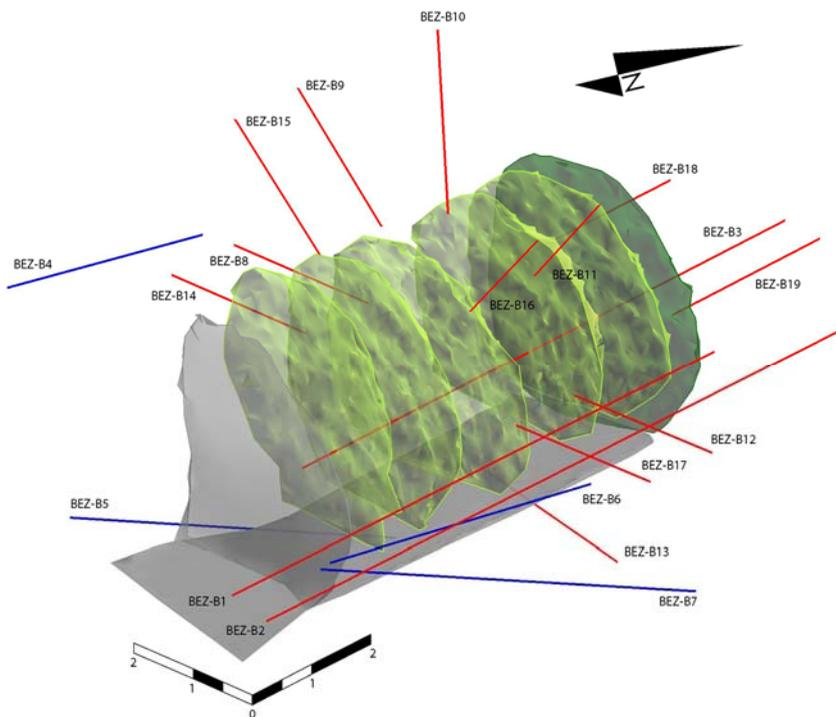
Fig. 2. An isometric view of the EZ-B niche construction and the borehole layout (drawing scale in metres). The entrance face is depicted in grey, the intermediary excavation steps in yellow, and the final face in green. The pore pressure boreholes are in blue and the observation boreholes in red. The top of the concrete floor is depicted in grey.
