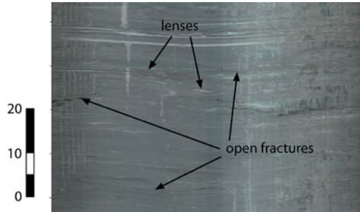
Fig. 6. Optical televiewer image (unwrapped) from a borehole drilled perpendicular to bedding. Sandy lenses and open fractures follow the bedding trace, which is subhorizontal. The scale is in centimetres.
