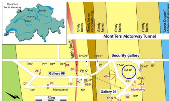
Fig. 1. The EZ-B experiment (circle) is located in the Mont Terri Rock Laboratory, Switzerland (inset).
