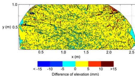
Fig. 9. A differential elevation map of the upper region of the final niche face that compares two laser scanning sessions six days apart (modified from Lemy *et al.*, in press).
