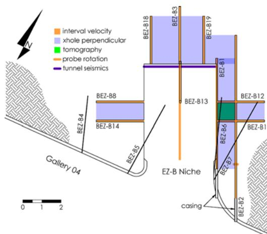
Fig. 8. Seismic measurements at the midheight of the niche (drawing scale in metres).
