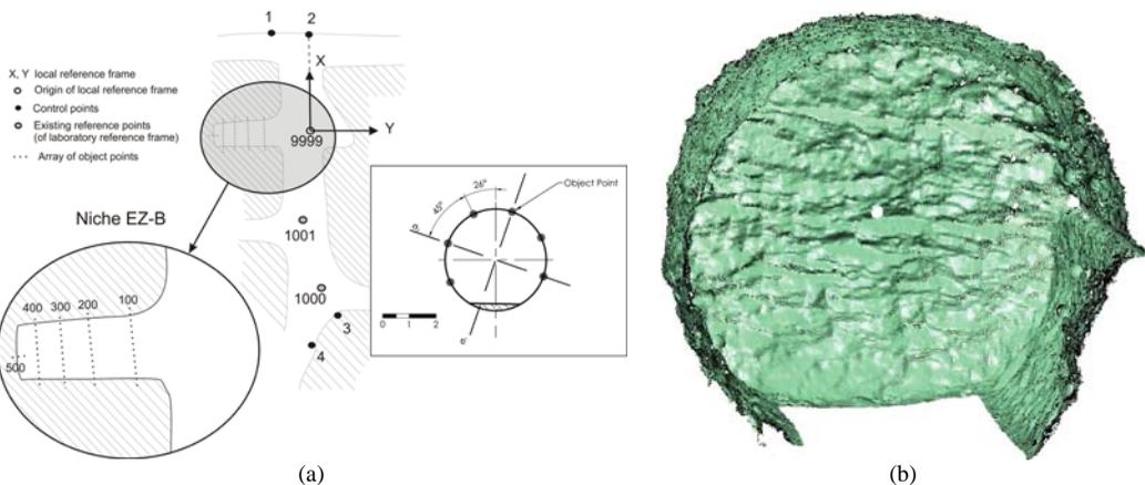
Fig. 7. The displacements were measured (a) at discrete points (inset) with a total station and along surfaces with a panoramic laser scanner via comparing point clouds (b). (modified from Lemy *et al.*, in press)
