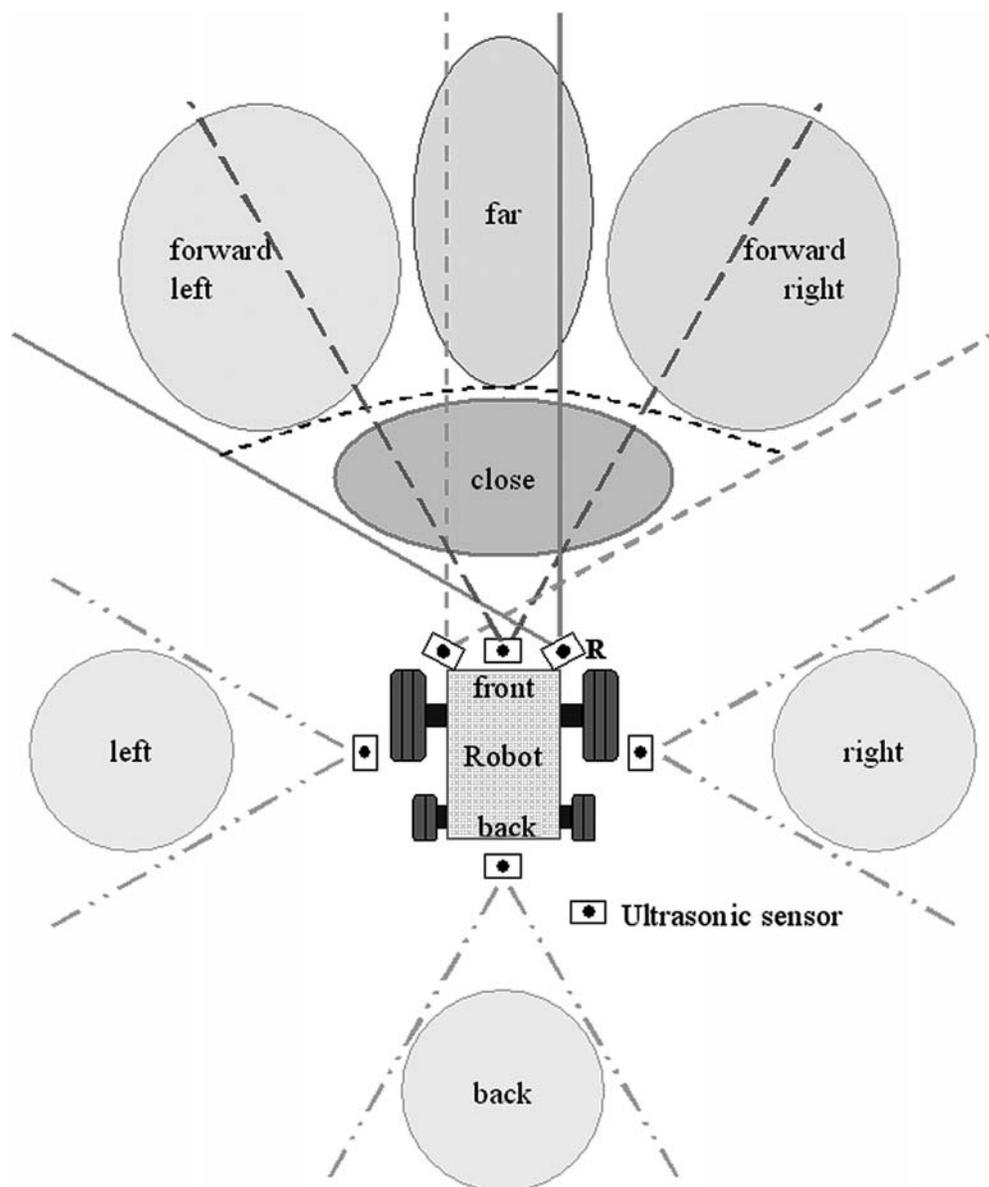
FIG. 7. A specific arrangement of six ultrasonic sensors.
