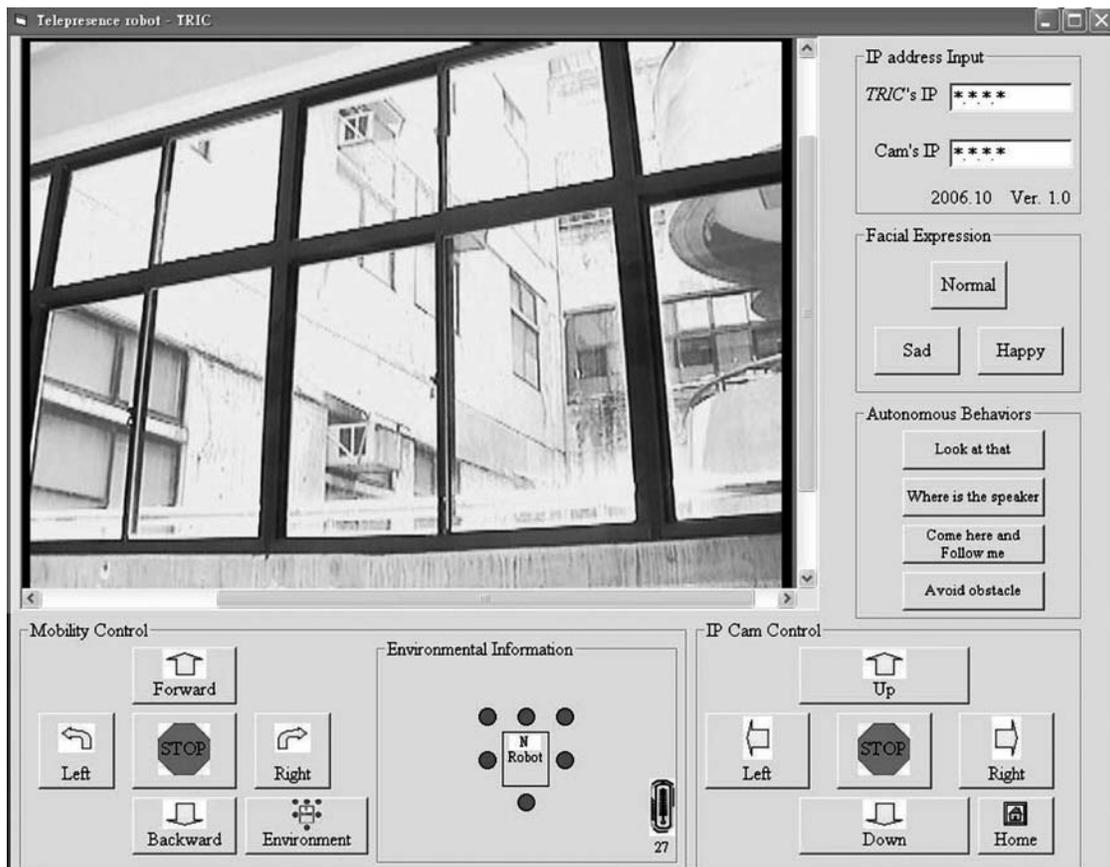
FIG. 8. Control interface for *TRIC*.
