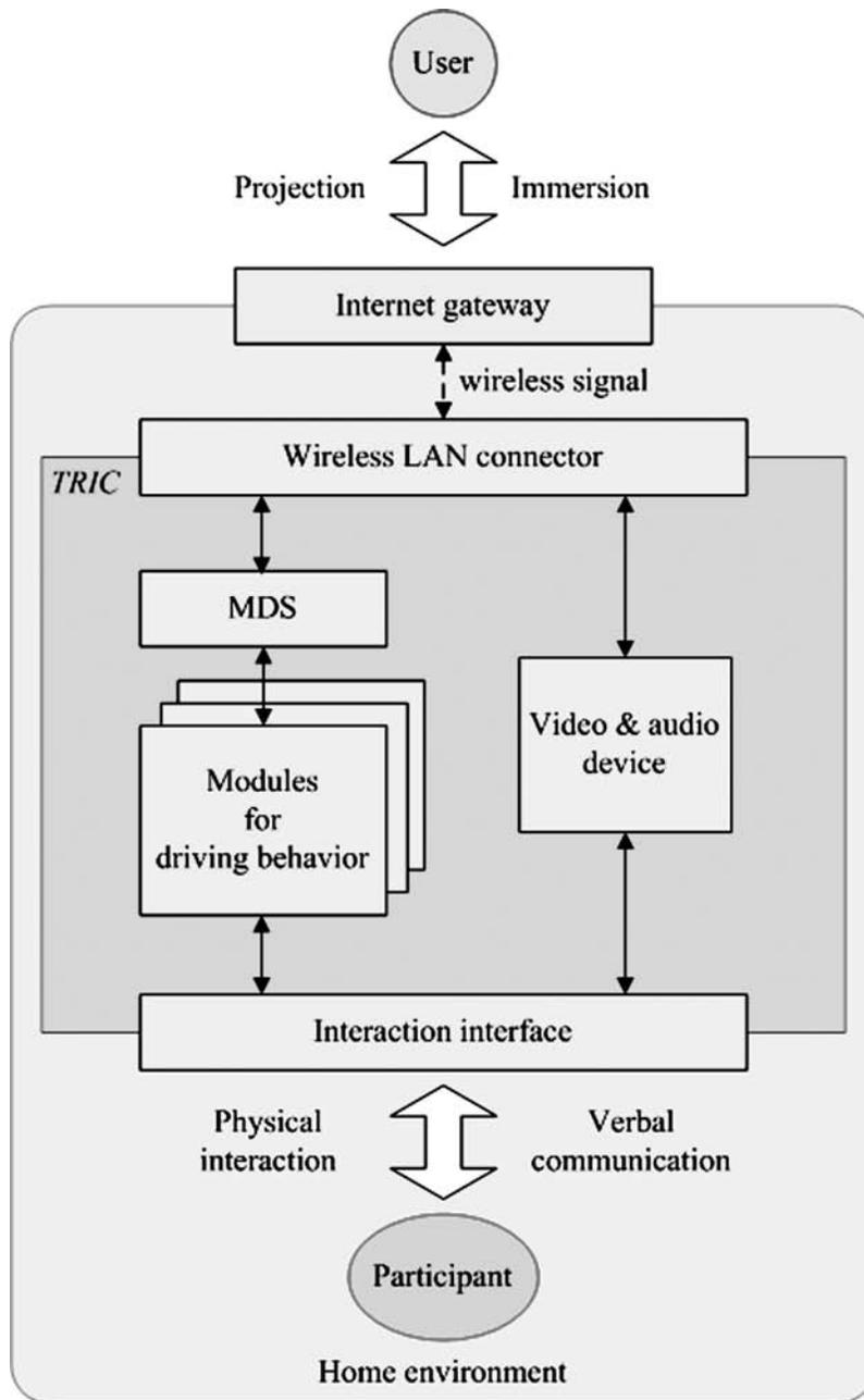
FIG. 3. The data transmission structure of TRIC.
