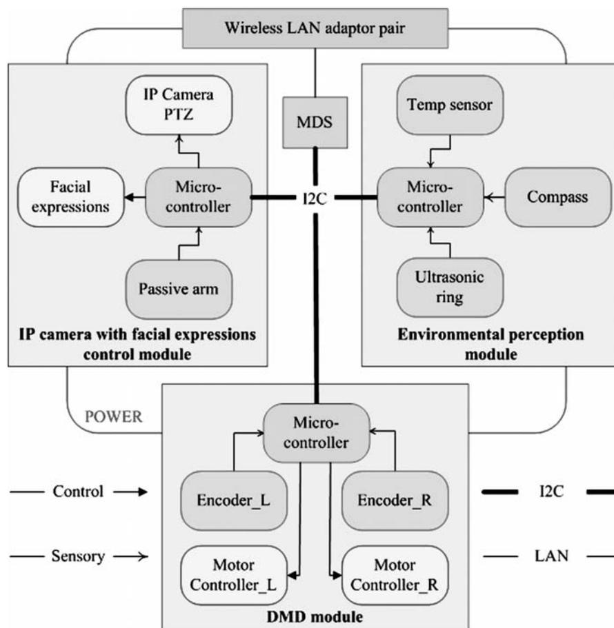
FIG. 6. Hardware architecture of the control system.
