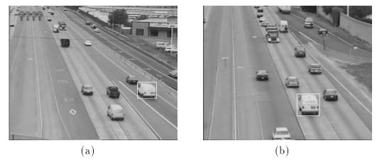
Fig. 1. Images from upstream (a) and downstream (b) surveillance cameras roughly two miles apart on Highway 99 in Sacramento, California. The boxed vehicle has been identified at both cameras.
