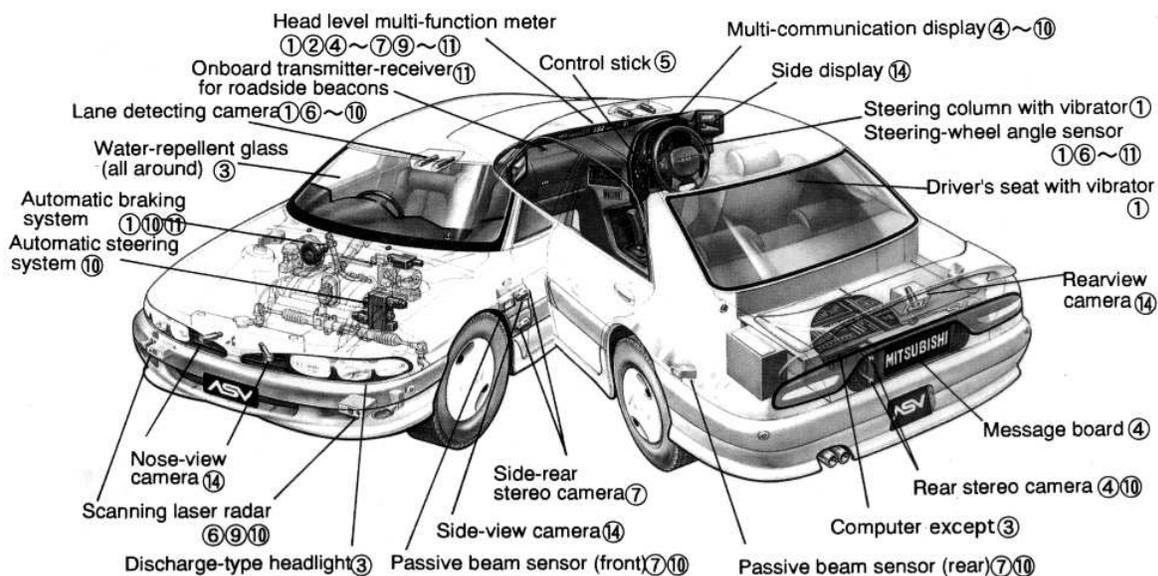
Figure 1: Main equipments of active safety
