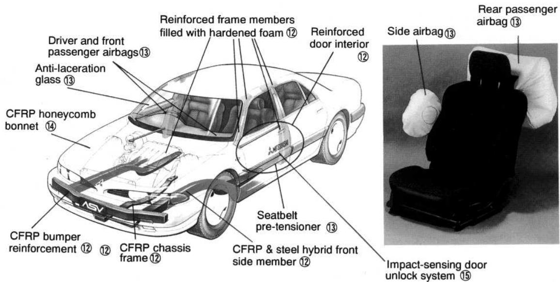
Figure 2: Main equipments of passive safety
