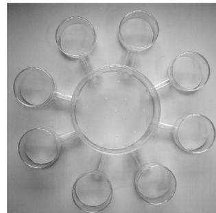
**Figure 1. A modified eight-chamber-olfactometer used for the food preference experiment. Cockroaches were placed in the center arena and allowed access to food choices in eight peripheral chambers (modified from Reiersen 1995).<sup>(8)</sup>**
