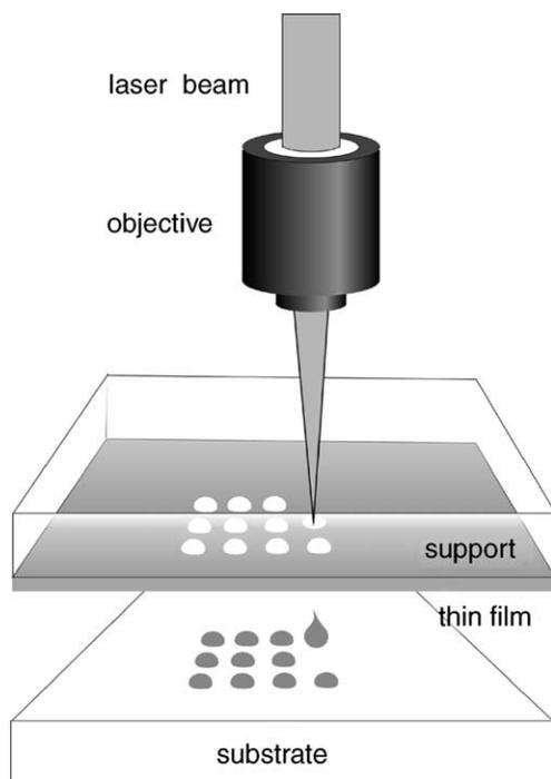
Fig. 1. Laser induced forward transfer scheme.
