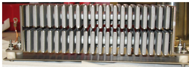
Figure 4: NEG module for installation inside the 150 l pump.
