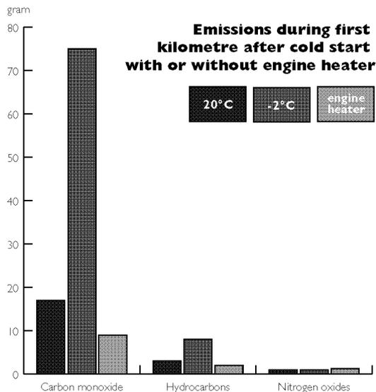
**Emissions at 20°C and -2°C with and without engine heater. Data for six cars with catalytic converters. Source: MTC report 9001.**
