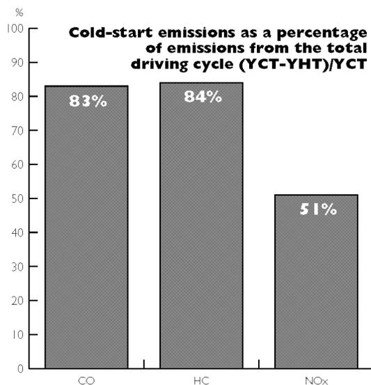
**Cold start emissions as a percentage of total emissions in the driving cycle. Data for average car, 1989 model. Source: ScanTech and MTC.**
