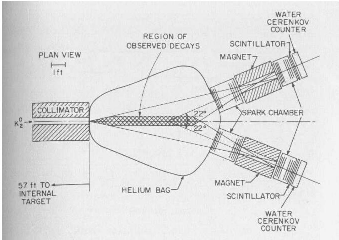
Figure 2: **Details of the spectrometer.** Taken from [3, p.123].
