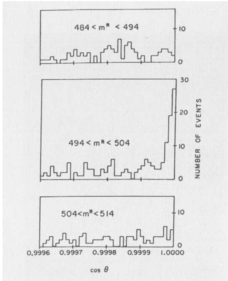
Figure 3: **Key evidence for  $CP$  violation.** This figure was taken from [3, p.130]. It was also included in the original paper [1]. It shows angular distribution in three mass ranges for events with  $\cos \theta > 0.9995$ . Note the sharp peak at  $\theta = 0^\circ$  for the mass range corresponding to the mass of the  $K_L$  (498 MeV).
