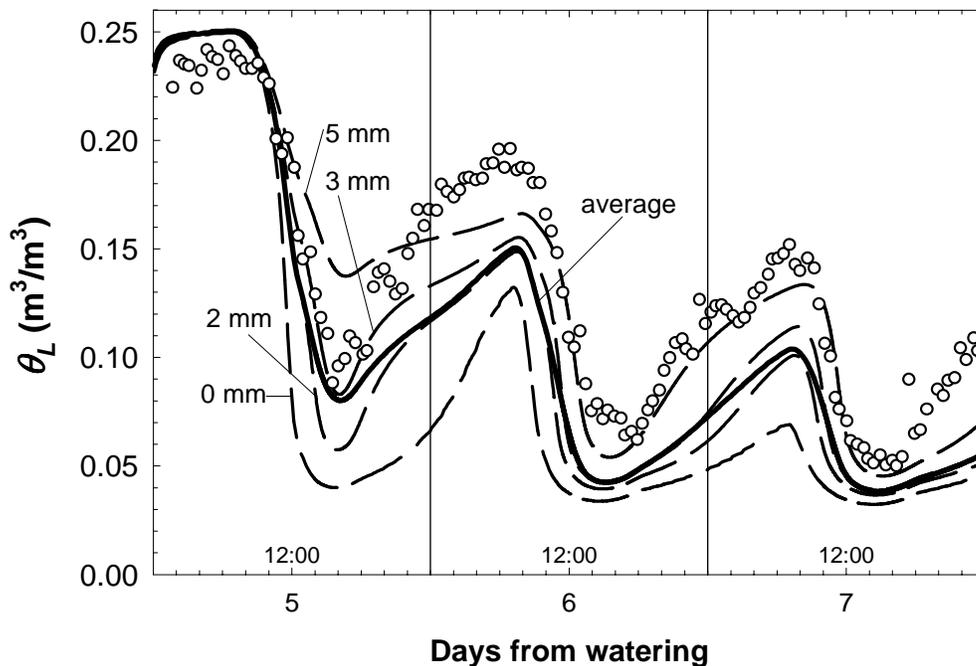
**Figure 6.** Simulations of the influence of wind speed and relative humidity on the integral average moisture content in the top soil layer (0-5 mm) for Test case II. The open symbols represent the experimental data of Jackson (1973).
