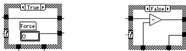
Figure 15: A LabVIEW conditional from the rocket program, showing both arms. In the LabVIEW environment, only one arm is visible on screen at any one time.
