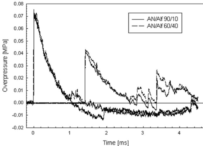
**Figure 3.** Overpressure profiles of incident blast waves for AN/Alf mixtures.
