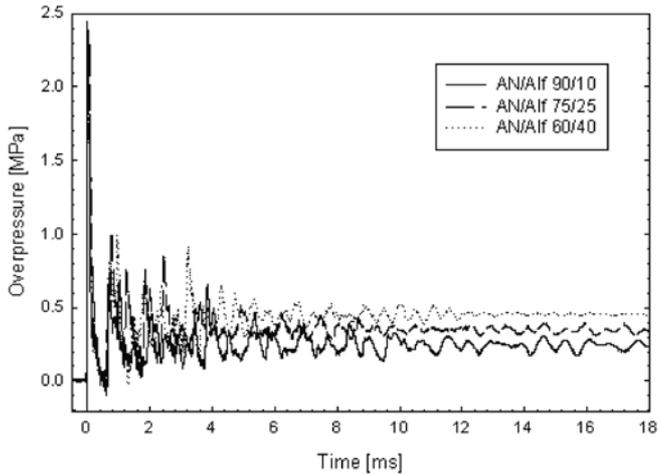
**Figure 1.** Exemplary overpressure histories recorded in the 0.15 m<sup>3</sup> chamber for ammonium nitrate/Alf mixtures.
