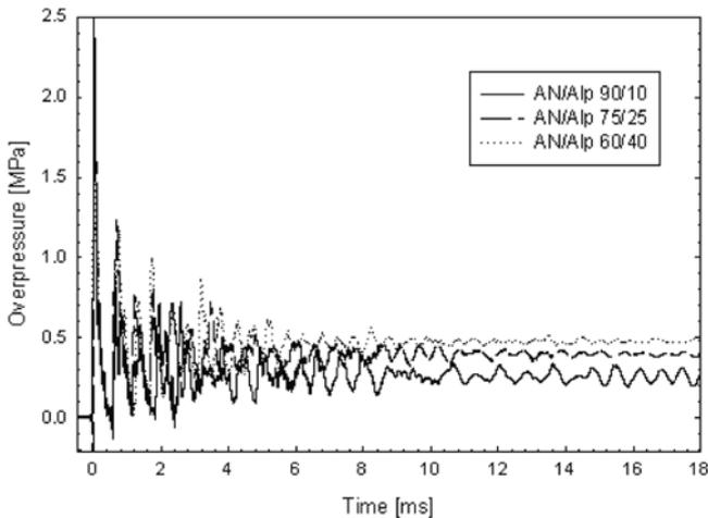
**Figure 2.** Exemplary overpressure histories recorded in the 0.15 m<sup>3</sup> chamber for ammonium nitrate/Alp mixtures.
