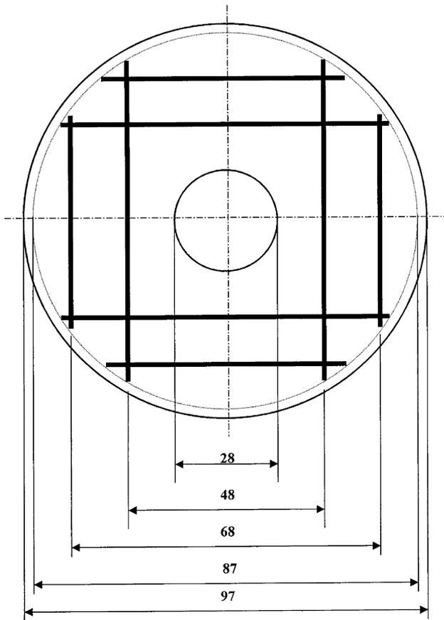
Fig. 2. Annular configuration of mortar reinforced with steel rebars (thick lines) for EMI shielding effectiveness testing. All dimensions are in millimeters.
