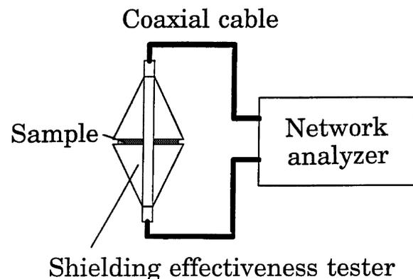
Fig. 1. EMI shielding effectiveness testing setup.
