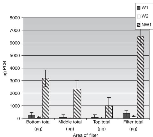
**Figure 7. PCB ( $\mu\text{g}$ ) in geotextile filters**
