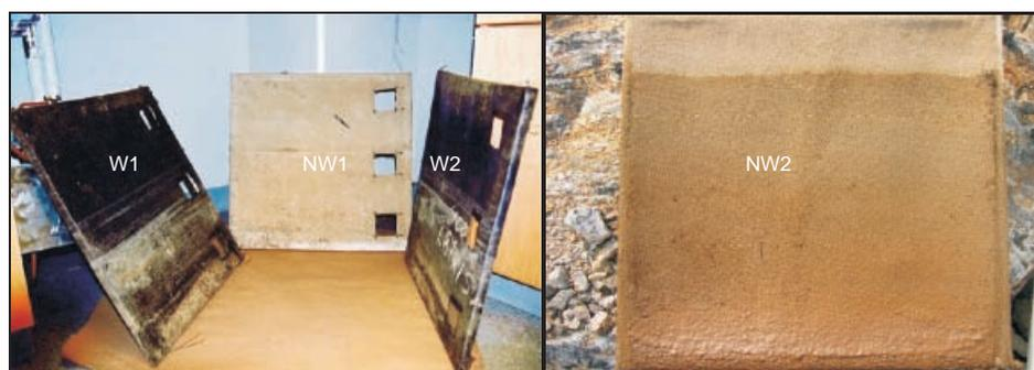
Figure 6. Geotextile filters used in 2003. Note soil stains
