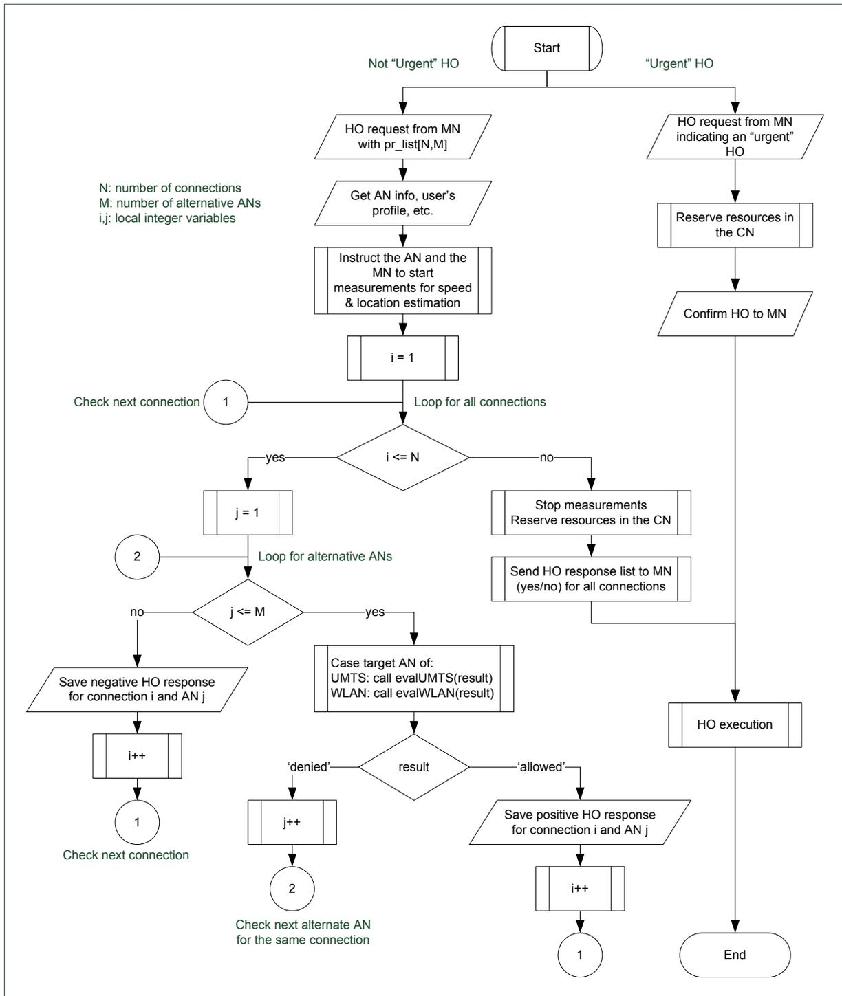
Fig. 4. Algorithm running in the core network
