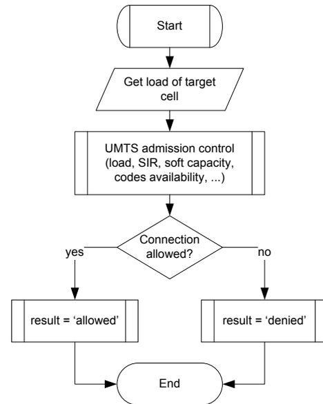
Fig. 5. Handover evaluation procedure in UMTS
