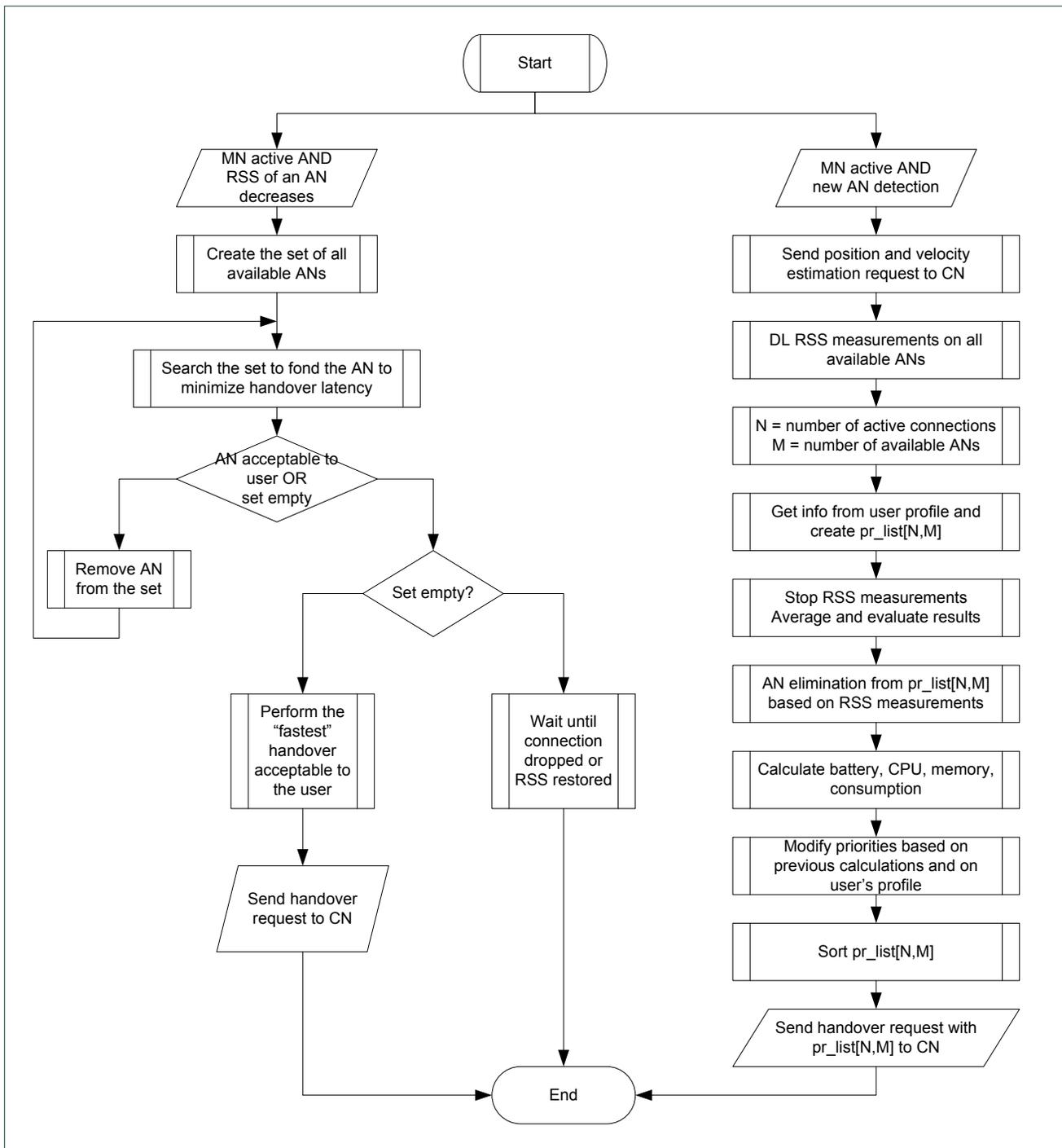
Fig. 3. Algorithm running in the mobile node
