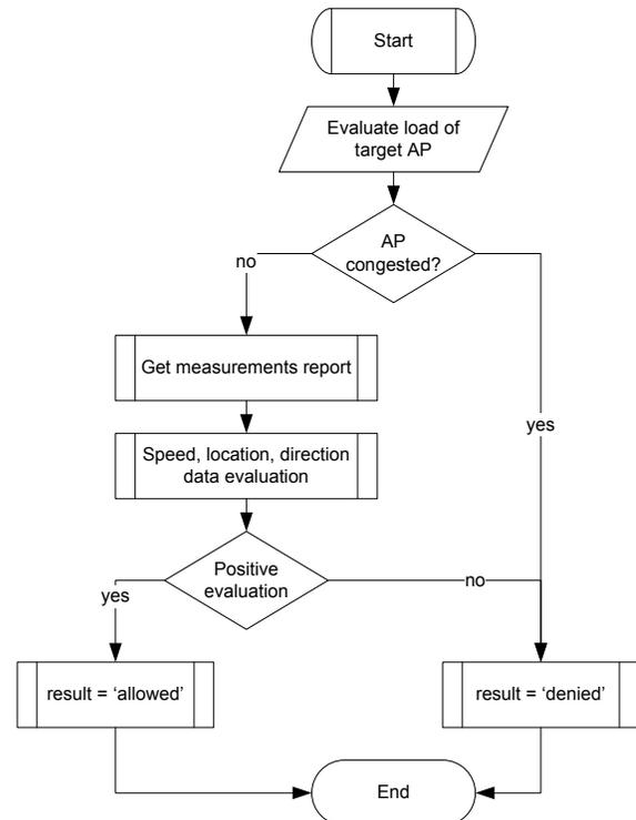
Fig. 6. Handover evaluation procedure in WLAN
