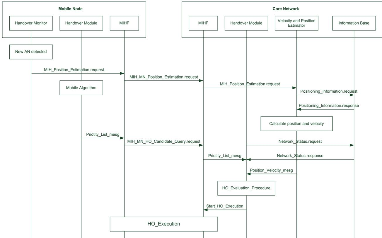
Fig. 7. Handover evaluation procedure in WLAN
