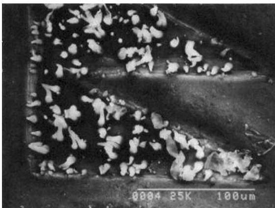
Fig. 8. The electroless copper nucleation grown in pattern that wetting by SDS before activation and acetone-cleaning after activation.
