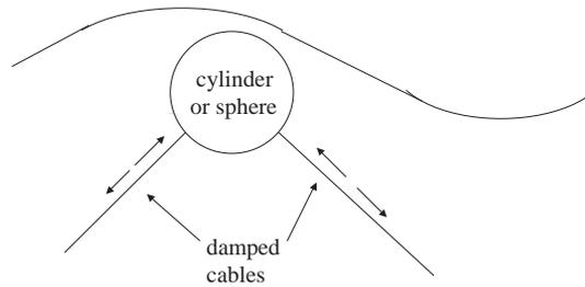
Fig. 2. The “Bristol cylinder” wave energy device.
