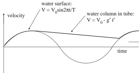
Fig. 3. Vertical velocity of water surface and water in tube.
