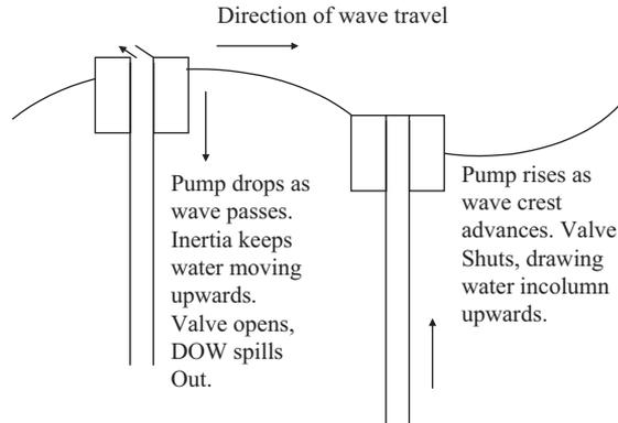
Fig. 1. Inertia pump action.
