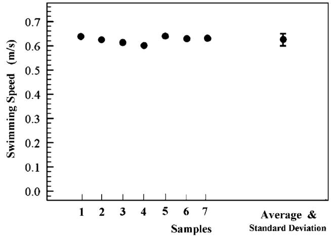
Fig. C.1. Swimming speed of seven examples is plotted at the left. Average speed with standard deviation is also shown at the right. The value of speed is  $v = 0.62 \pm 0.01$  m/s. This graph shows small fluctuation among samples and small standard deviation.
