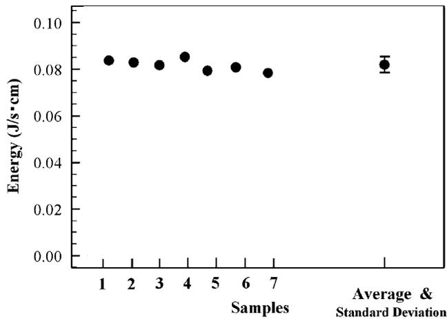
Fig. C.3. Averaged energy for each sample is plotted at the left. Average energy over seven samples is shown with standard deviation at the right. The energy is calculated as  $0.082 \pm 0.002$  J/(s cm). Small standard deviation is also observed from this figure.
