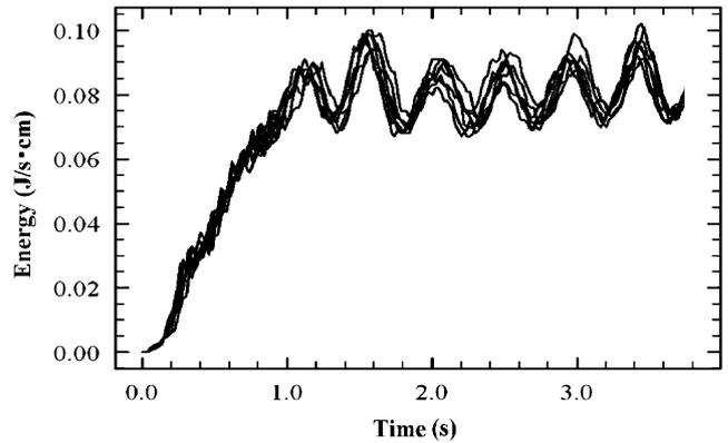
Fig. C.2. Energy profile of seven different swimming motion. Initial stage from 0 to 1.2 s shows transition from the rest position to steady state swimming motion. The later process shows steady state of swimming motion of model *Anomalocaris*. Oscillatory pattern of energy profile is caused by waving motion of the lobe of model *Anomalocaris*.
