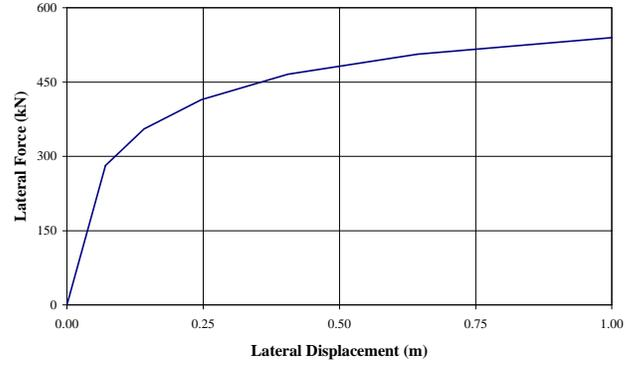
Fig 4: Force / Displacement for Buried Pipeline
