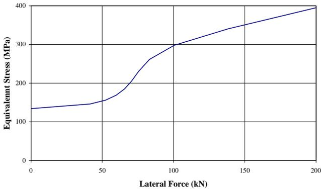
Fig 2: Force / Equivalent Stress for Pipeline on Surface
