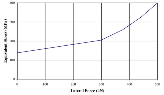
Fig 5: Force / Equivalent Stress for Buried Pipeline
