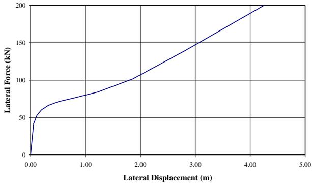
Fig 1: Force / Displacement for Pipeline on Surface
