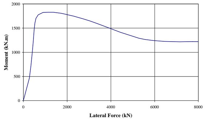
Fig 6: Moment / Force Stress for Buried Pipeline
