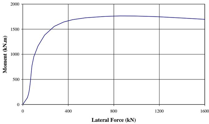
Fig 3: Moment / Force Stress for Pipeline on Surface
