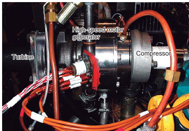
Fig. 5 Conditions of the test on the hybrid turbo, and the external appearance of the motor stator Hybrid turbo during the engine testing. A 6-slot concentration winding method is adopted for the motor stator to downsize the component and reduce loss.
