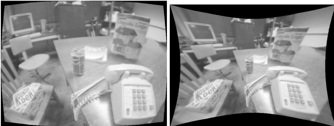
Figure 9: In stereographic projection (left), the shape of an object is approximately the same, regardless of where it occurs in the field of view, unless it subtends a large visual angle. In perspective projection (right), objects near the periphery (e.g. the phone) are visibly distorted.
