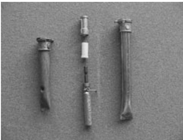
**Fig. 3.** The "Poteet" model M-44 as made at Pocatello Supply Depot from approximately 1969 through 1984. From lower left, a 5-inch Leyerly top stake, ejector, polyethylene M-44 cyanide capsule, capsule holder, and 7-inch Leyerly top stake.
