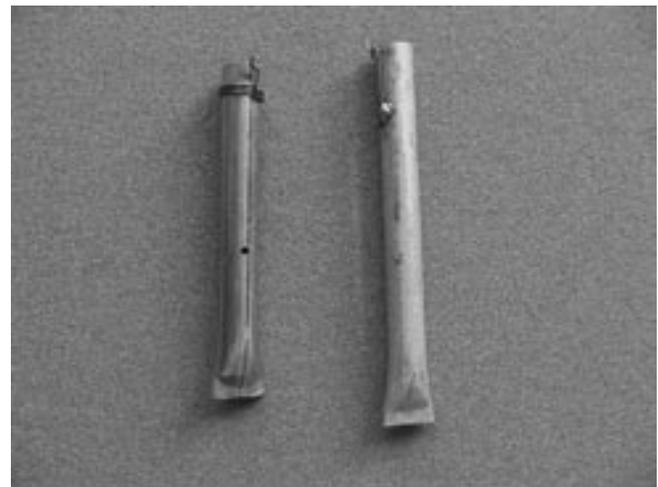
**Fig. 9. Prototype of an M-44 stake designed by PSD Manager Paul Edstrom (1988). The Edstrom stake (left) featured an ejector retaining clip that was modeled after the wire clip on the much earlier coyote getter stake (right).**
