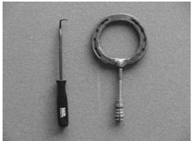
**Fig. 11. M-44 stake pullers. From left, cotter-pin extractor tool modified by Montana ADC Specialist Denny Biggs and the 'horseshoe' tool developed by Arizona ADC Specialist J. Brad Miller. Both tools were introduced in 1996.**
