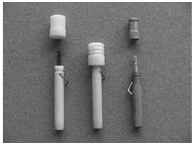
**Fig. 4. Prototype plastic M-44 ejectors (left and center), hand made by Nebraska ADC Specialist Don Thalheim about 1982. The ejector bodies were machined to accommodate stock M-44 metal plungers, triggers and ejector springs. A standard M-44 ejector and capsule holder (Edstrom model, ca. 1985) are shown at right for comparison.**
