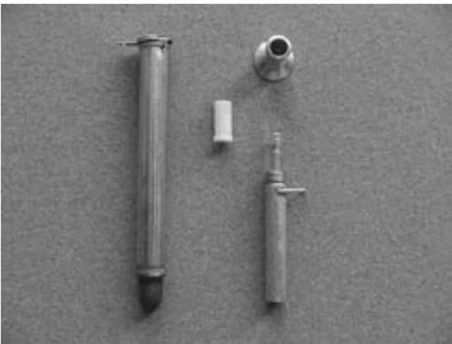
**Fig 7. Current production (2002) M-44 equipment from Pocatello Supply Depot. From left: stake, polyethylene M-44 cyanide capsule, Edstrom-style ejector with retaining pin, and capsule holder with lip to deflect precipitation from running into the stake.**
