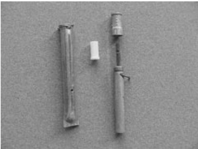
**Fig. 5. The Keenan model M-50 cyanide ejector as made at Pocatello Supply Depot during 1979-1983. From left: 6-inch swaged-top stake, polystyrene cyanide capsule, ejector, and capsule holder.**
