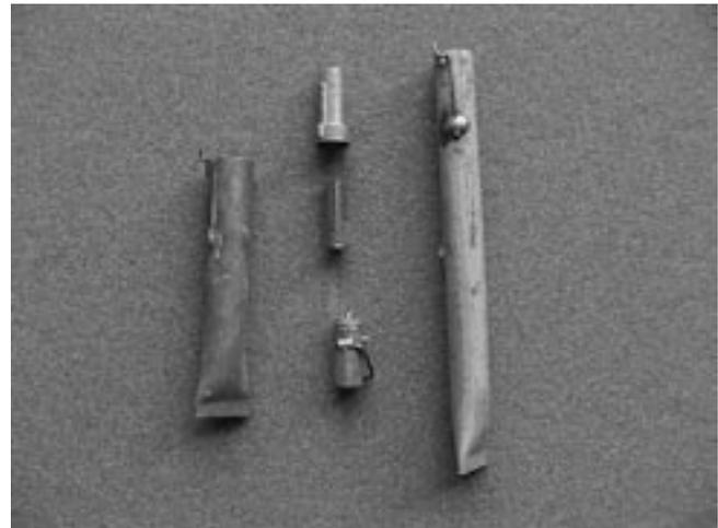
**Fig. 1. Coyote getter as used by government hunters before 1970. From lower left: 5-inch stake, firing unit, cyanide shell, shell holder, 7-inch stake.**
