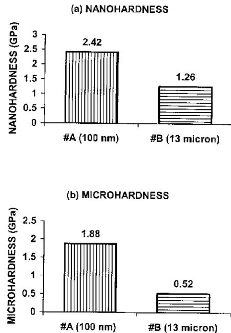
Fig. 5. Bar graph comparing the hardness of the two copper samples: (a) nanoindentation, and (b) microhardness.
