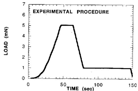
Fig. 2. A typical load–time sequence (peak load = 120 mN).
