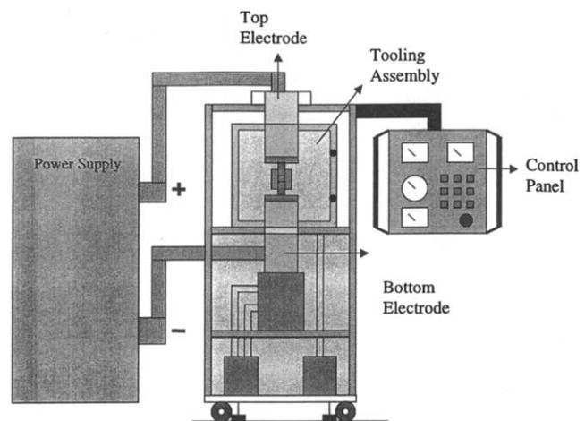
Fig. 1. A schematic of the plasma pressure consolidation (P<sup>2</sup>C) set up.
