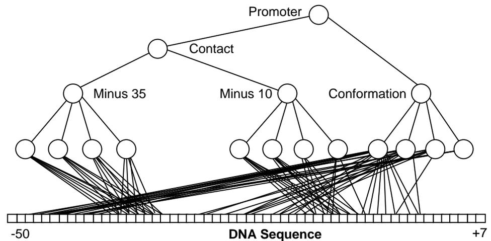
**Figure 8** The initial KBANN-net for promoter recognition (low-weighted links are not shown). Each box at the bottom of the figure represents one sequence location which is encoded by four input units.
