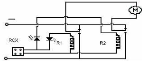
**Figure 9 Relay motor controller for RCX**
