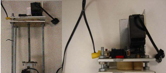
**Figure 7 Electromechanical ballast system**
