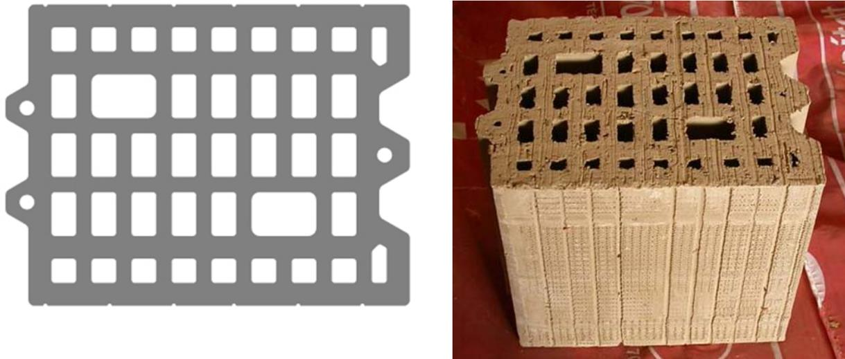
Figure 3 Shape of the newly developed unfired clay block
