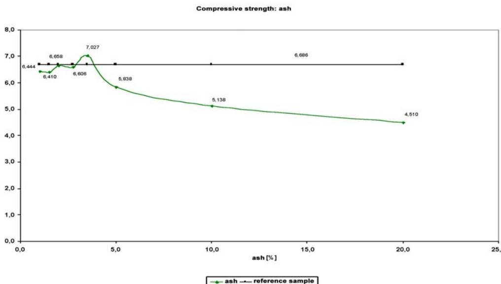
Figure 2 Example: influence of wood ash as additive on the compressive strength of the loam
