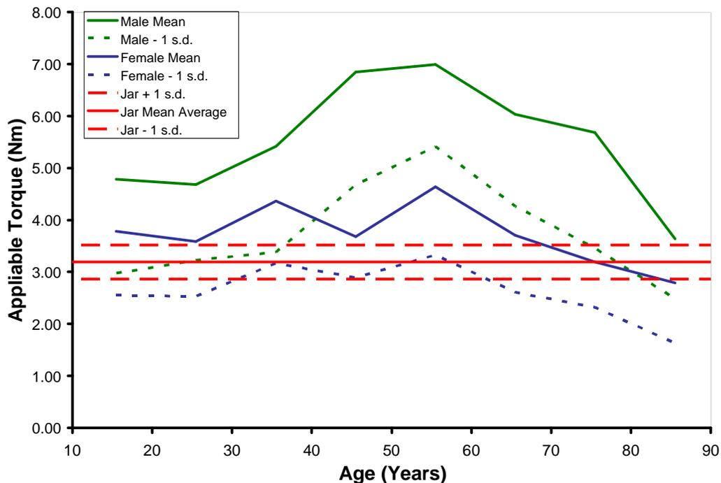
Figure 2. Graph of mean applicable torque against age for 75mm vacuum lug closure.
