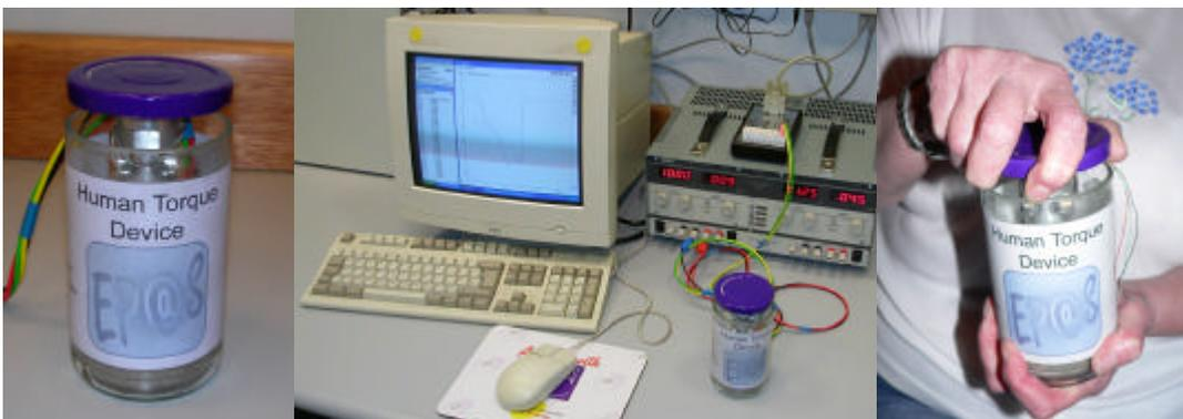
Figure 1. Photographs of the torque device (left), the test equipment (centre) and the device in use during a test (right).
