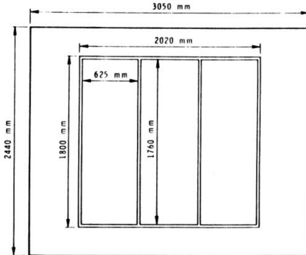
Figure 2: Location and size of window openings in the filler wall.
