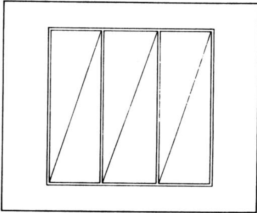
Figure 4: View of test wall from either reverberation room to indicate location of diagonal dividers in interpane cavities
