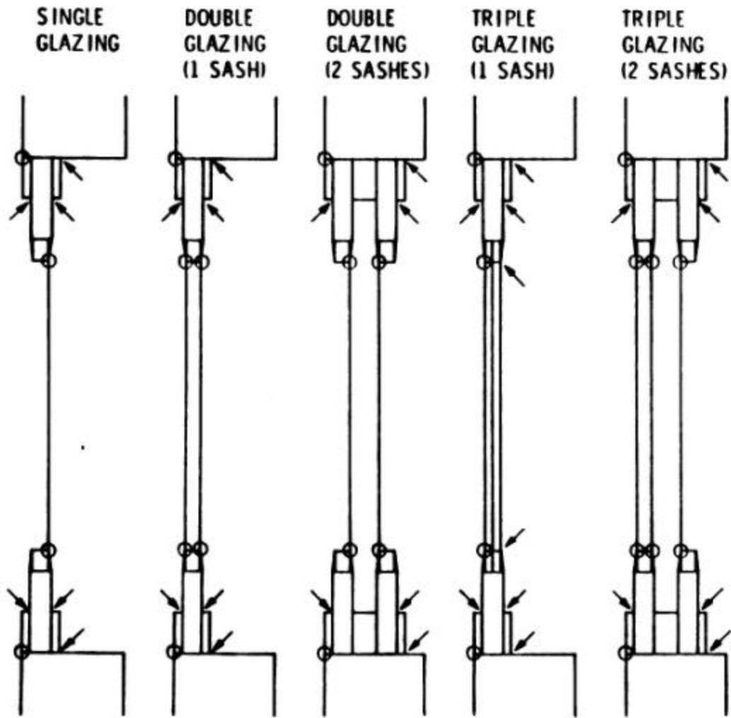
Figure 3: Schematic representation of window mounting details. caulked seals are indicated by circles, and taped seals are indicated by arrows
