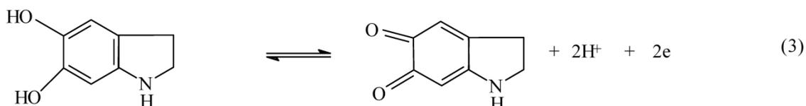
**Scheme 1.** Proposed DA reactions at poly(3-acetylthiophene)/GCE in 0.1 M PBS at pH 7.2.
