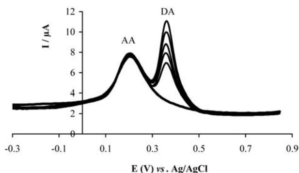
**Fig. 7.** Square wave voltammograms of the mixture of various concentrations of DA in the presence of  $2.5 \cdot 10^{-4}$  M AA at poly(3-acetylthiophene)/GCE. DA concentrations:  $1.25 \cdot 10^{-5}$  M,  $1.5 \cdot 10^{-5}$  M,  $2.0 \cdot 10^{-5}$  M,  $2.25 \cdot 10^{-5}$  M and  $2.75 \cdot 10^{-5}$  M. Equilibrium time: 5 s, frequency: 10 Hz, step potential: 20 mV, amplitude: 25 mV.
