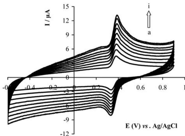
**Fig. 3.** Cyclic voltammograms of  $2.5 \cdot 10^{-5}$  M DA at poly(3-acetylthiophene)/GCE in 0.1 M PBS at pH 4.0. Scan rates: (a) 50 mV/s (b) 75 mV/s (c) 100 mV/s (d) 125 mV/s (e) 150 mV/s (f) 175 mV/s (g) 200 mV/s (h) 225 mV/s (i) 250 mV/s. Equilibrium time: 5 s.
