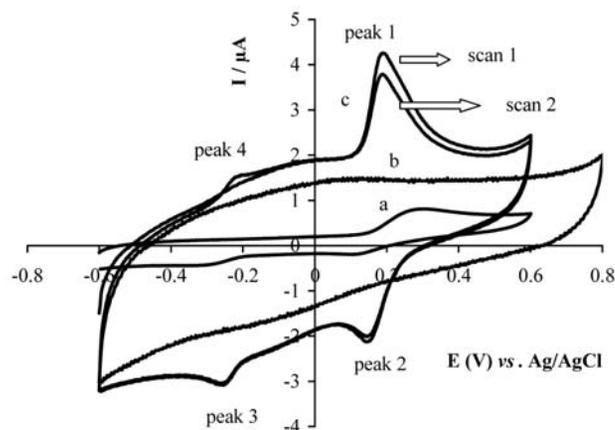
**Fig. 1.** Cyclic voltammograms of (a)  $2.0 \cdot 10^{-5}$  M DA at bare GCE (b) poly(3-acetylthiophene)/GCE and (c)  $2.0 \cdot 10^{-5}$  M DA at poly(3-acetylthiophene)/GCE. Supporting electrolyte: 0.1 M PBS at pH 7.2. Equilibrium time: 5 s, scan rate: 50 mV/s.
