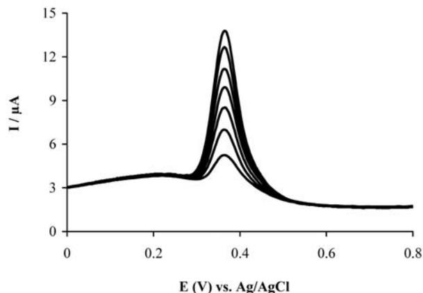
**Fig. 5.** Square wave voltammograms of increasing concentration of DA at poly(3-acetylthiophene)/GCE in 0.1 M PBS at pH 4.0. DA concentrations:  $5.0 \cdot 10^{-6}$  M,  $1.0 \cdot 10^{-5}$  M,  $1.5 \cdot 10^{-5}$  M,  $2.0 \cdot 10^{-5}$  M,  $2.5 \cdot 10^{-5}$  M,  $3.0 \cdot 10^{-5}$  M,  $3.5 \cdot 10^{-5}$  M. Equilibrium time: 5 s, frequency: 10 Hz, step potential: 20 mV, amplitude: 25 mV.
