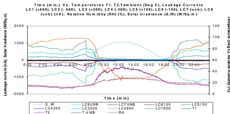
Figure 6: Variation of leakage current, solar irradiance, temperatures, and relative humidity versus time of day.
