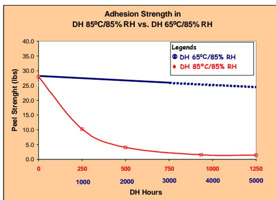
**Figure 5:** Adhesion of back sheet to EVA after testing at 85°C/85% RH and 65°C/85% RH.
