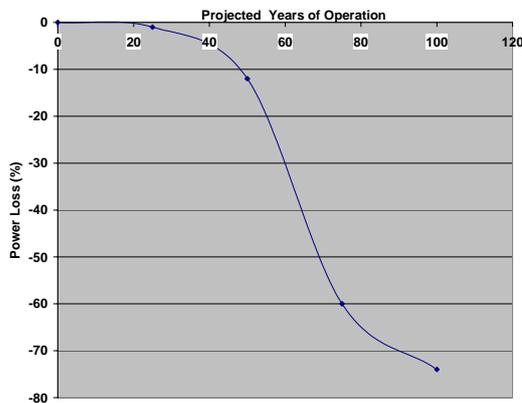
**Figure 4:** Projected Long Term Performance of Module Based on Damp Heat Testing
