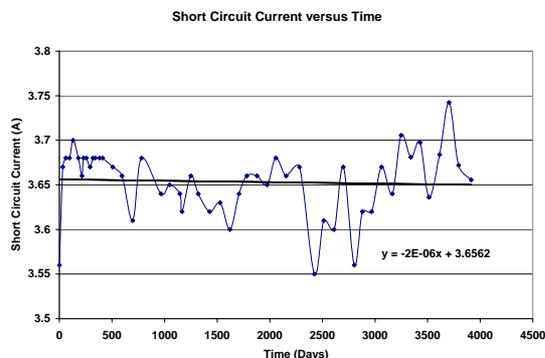
Figure 2: Change in Short Circuit Current for one module fielded in Arizona for more than 10 years.
