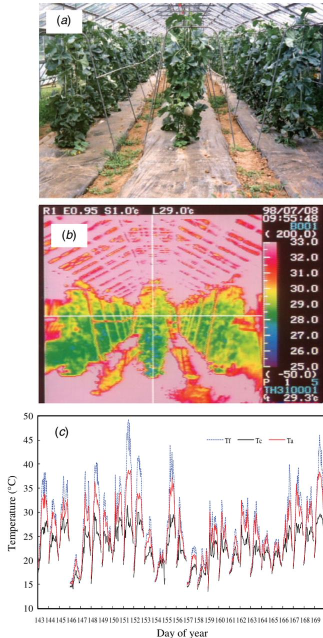
**Fig. 1.** Glasshouse experiment with melon plants. (a) The experiment arrangement and (b) the corresponding thermal image on 8 July 1998. (c) Variation of the three temperatures in day of year (DOY) 143–169, where  $T_c$  is the temperature of the melon leaf,  $T_f$  is the temperature of the dry reference leaf and  $T_a$  is the temperature of the air.
