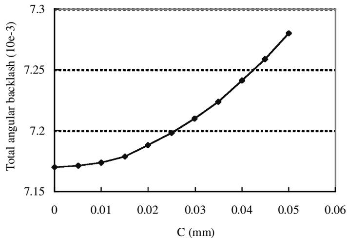
**Fig. 5** Minimum total angular backlash versus the change in centre distance tolerance
