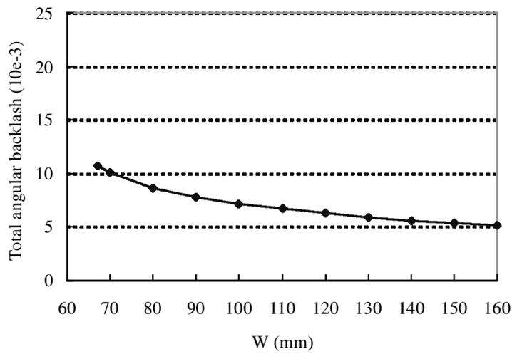
**Fig. 3** Minimum total angular backlash versus the change in available space
