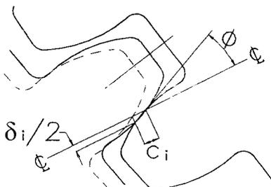
Fig. 2 The influence of centre distance tolerance on gear backlash
