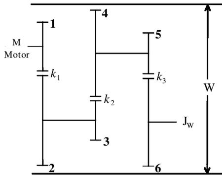
Fig. 1 A three-stage gear transmission system
