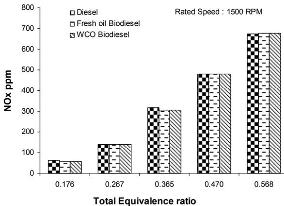
Figure 6. NOx emission versus total equivalence ratio
