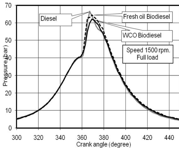
Figure 3. Pressure versus crank angle diagram for the three test fuels
