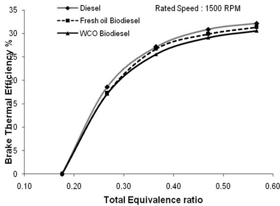
Figure 2. Brake thermal efficiency versus total equivalence ratio
