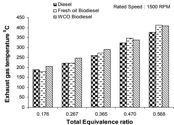
Figure 5. Exhaust gas temperature versus total equivalence ratio
