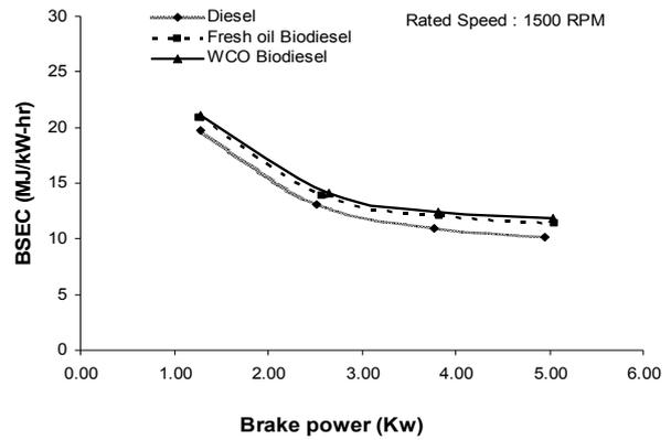
Figure 4. BSEC versus brake power developed for the three test fuels
