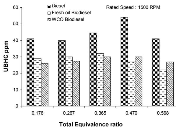
Figure 7. UBHC emission versus total equivalence ratio
