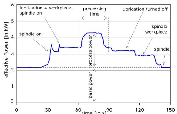
Figure 3: Energy Profile of a production machine (e.g. grinding process) [7]
