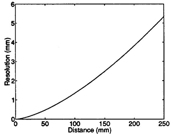
**Figure 6.** Proximity resolution of a surrogate arm in shunt mode plotted as a function of distance from dipole to arm. Resolution is the change in distance that produces a 6dB change in signal over noise.
