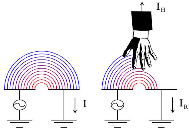
**Figure 1.** An electric dipole field created between an oscillating transmit electrode and virtual ground receiver electrode is intercepted by a hand. Displacement current to ground  $I_R$  decreases as the hand moves further into the dipole field.
