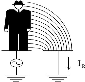
**Figure 2.** Energy from an oscillator is coupled into a person standing on the transmit electrode making the person an electric field emitter. As the person moves any body part closer to the grounded receive electrode, the displacement current into the receiver  $I_R$  increases.
