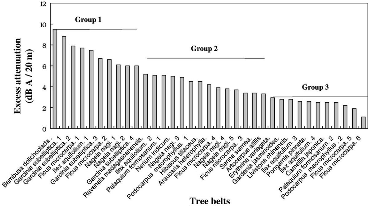
Fig. 5. The excess attenuation of 35 tree belts.
