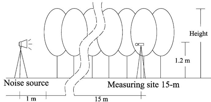
Fig. 4. The profile of experimental design.
