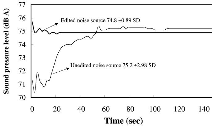
Fig. 2. The accumulative mean value of sound pressure level from the edited and unedited noise source.
