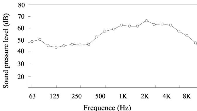
Fig. 1. One-third octave band center frequency at 5 m from the edited noise source.
