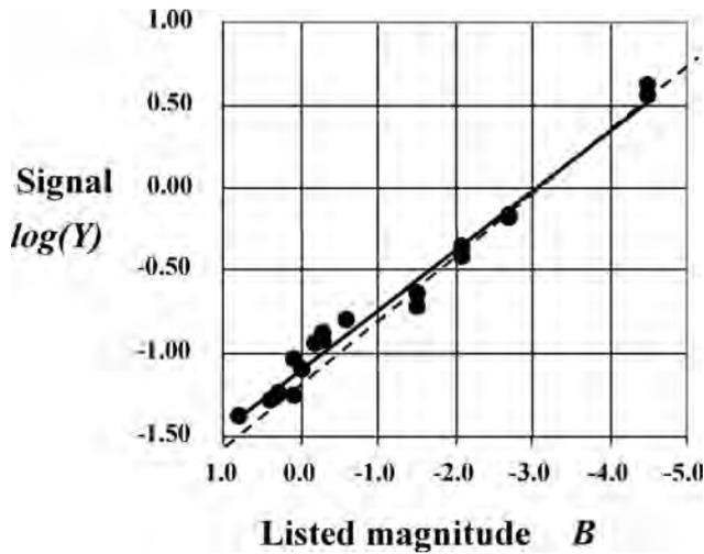
Fig. 1. Log-linearity of the LS-110 luminance photometer's scale for selected stars and planets (solid line, linear regression model; dashed line, same with unit brightness slope). Because these objects are essentially pointlike, the instrument's readings  $Y$  are not luminosities, but proportional to their luminous intensities.
