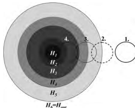
Fig. 5. Simplified geometry: the relative luminance within the umbra and penumbra is modeled by a disk plus a number of rings (here four) of certain width, each characterized by a constant normalized luminance (stepwise gray scale) of residual solar illumination. Four different positions of the Moon during the eclipse are shown (for details see text).
