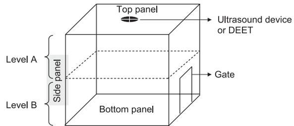
**Figure 1** Diagram of plexiglas chambers, used in experiments with mosquitoes, showing top, bottom, and side panels.
