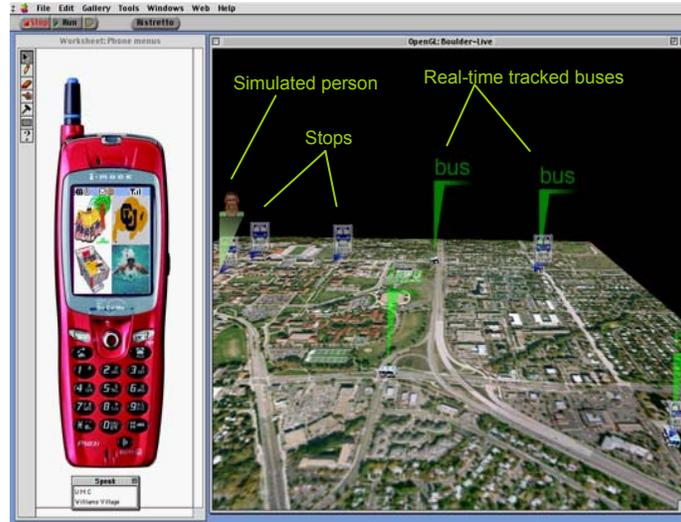
**Figure 2: Agent-based prototype showing a mobile prompting device synchronized with a virtual 3D display of real-time bus system.**
