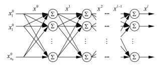
Fig. 1 A feedforward neural network
