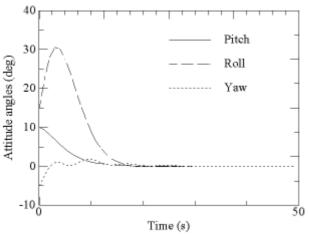
Fig. 6 – Attitude simulation with a PD controller
