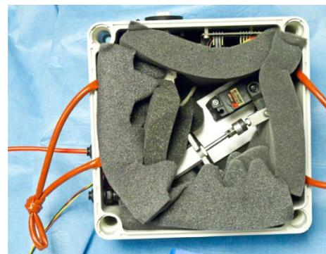
Figure 5-9 Left: First tactile prototype with rotating base. Right: The sound insulated servo driven hydraulic actuation unit. The device is hung underneath the force feedback hardware to eliminate audible vibrations.
