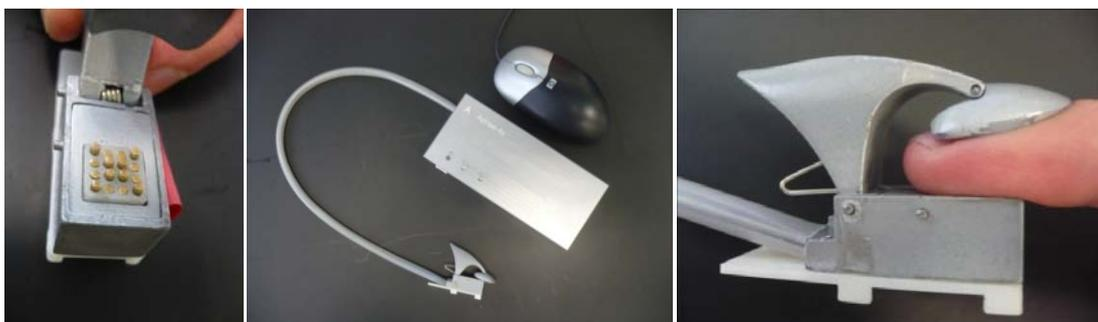
Figure 5-6 Finger mountable pin array device developed at Salford University [194].
