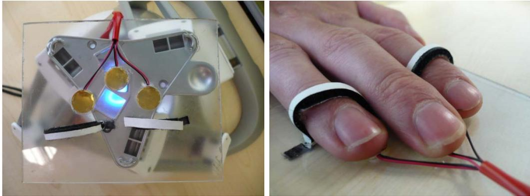
Figure 5-4. Left: Piezoelectric pads mounded onto a customised Falcon end effector. Right: The position of a user's fingertips on top of the modified end effector.
