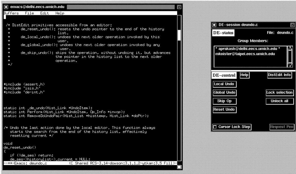
Figure 2: Sample screen display of a DistEdit-based group editor. The window on the right allows experimentation with the various undo facilities of DistEdit, such as per-user undo and global undo.
