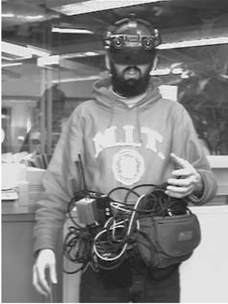
Figure 3: ‘Reality mediator’ as of late 1994, showing a color stereo head-mounted display (VR4) with two cameras mounted to it. The inter-camera distance and field of view match approximately my interocular distance and field of view with the apparatus removed. The components around my waist comprise radio communications equipment (video transmitter and receiver). The antennas are located at the back of the head-mount to balance the weight of the cameras, so that the unit is not front-heavy.
