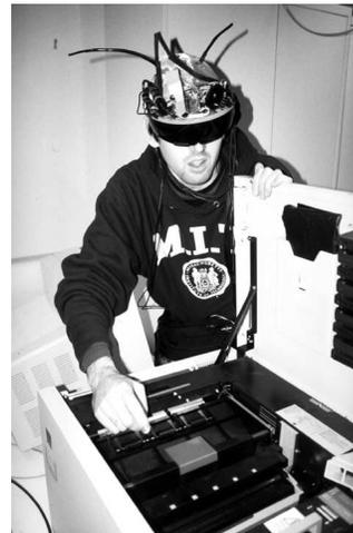
Figure 13: Equipment repair in a ‘mediated-reality’ environment. In this case, a laser printer is being serviced; note the colored tape installed in the printer and on my fingertip.
