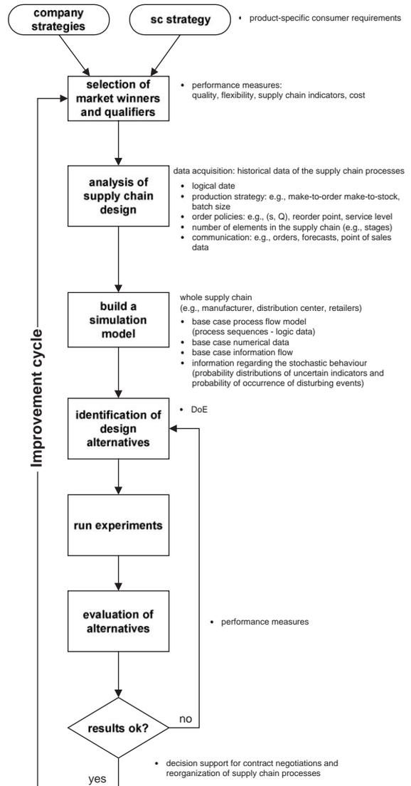
Fig. 1. Product-specific supply chain design model.
