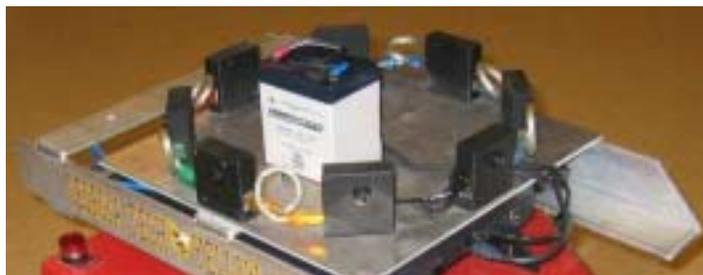
Fig. 15. Custom made camera rig, mounted on top of an ATRV-Mini mobile robot. Eight Fire-Wire cameras are distributed equally along a circle and connected to an on-board laptop.
