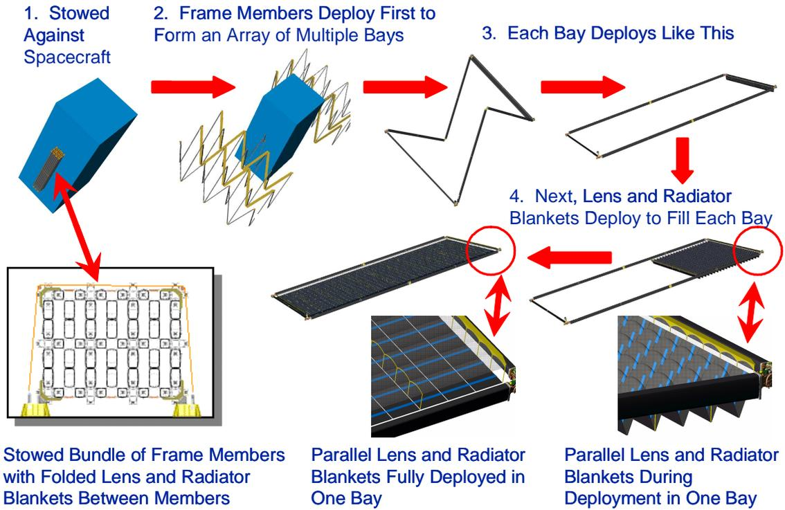
Figure 4. Stretched Lens Array SquareRigger (SLASR) schematic.
