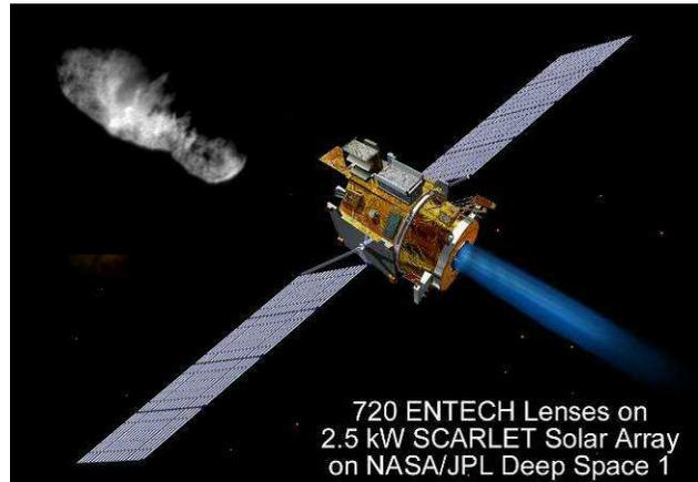
**Figure 2. SCARLET array on NASA/JPL Deep Space 1 probe (1998-2001).**
