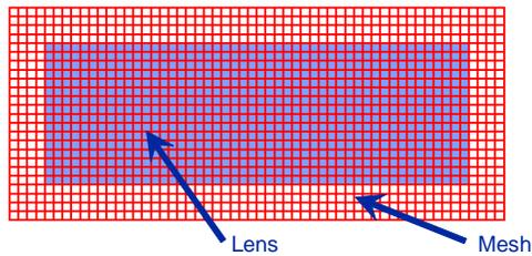
For High-Radiation Missions, a Thick (1-5 Microns) Parquet Coating, Using a Mesh During Deposition of the Thick Layer, Will Offer Additional Lens Radiation Hardness While Maintaining Lens Flexibility
