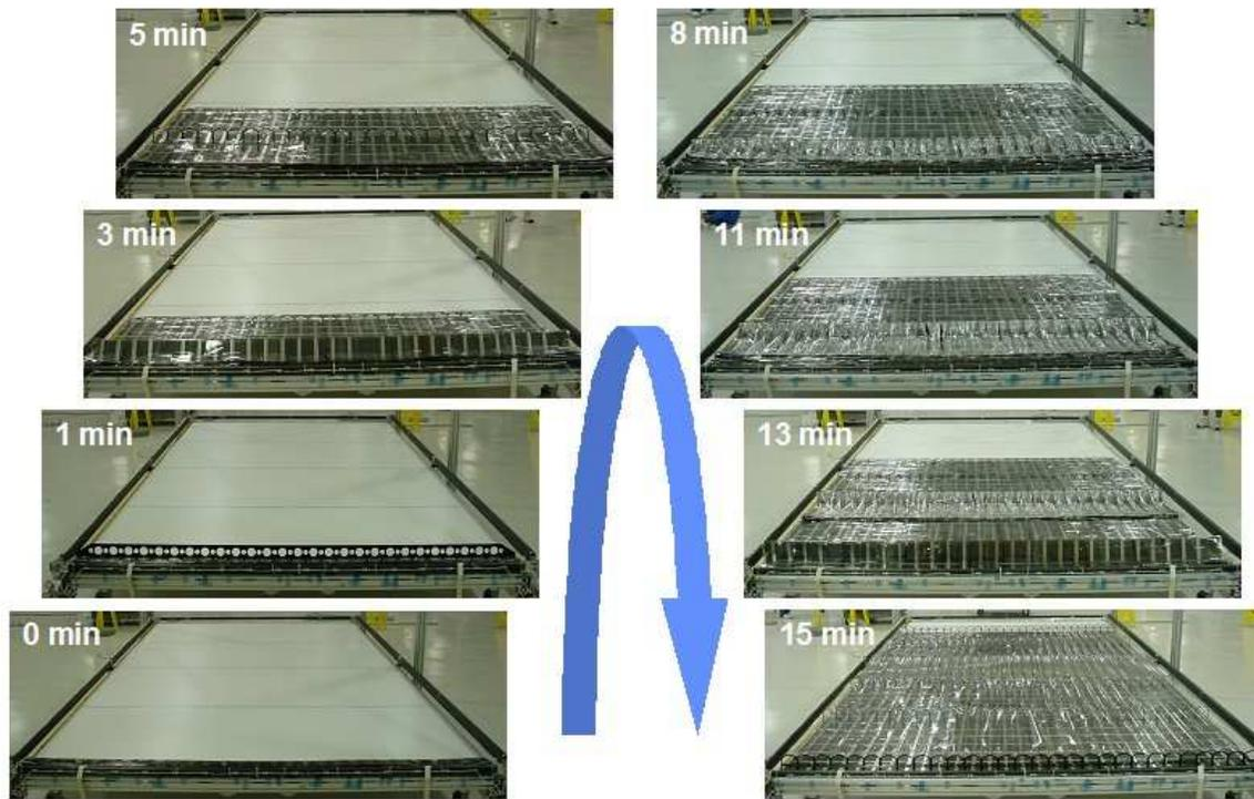
**Figure 6. SLASR lens and radiator blanket deployment.**
