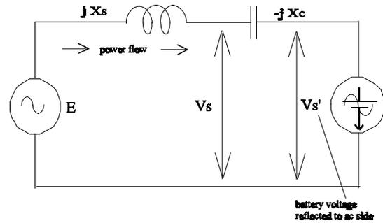
FIGURE 12. PER-PHASE EQUIVALENT CIRCUIT FOR SERIES COMPENSATED SYSTEM.
