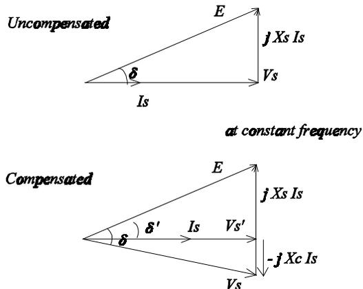
FIGURE 13. PHASOR DIAGRAM FOR SERIES CAPACITOR COMPENSATION
