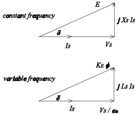
FIGURE 6. PHASOR DIAGRAMS OF AN UNCOMPENSATED SYSTEM.
