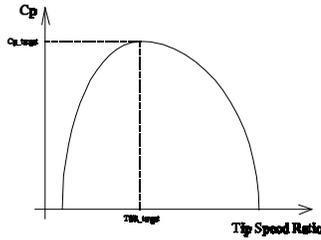
FIGURE 2. TYPICAL  $C_p$ -TSR CHARACTERISTIC OF A WIND TURBINE
