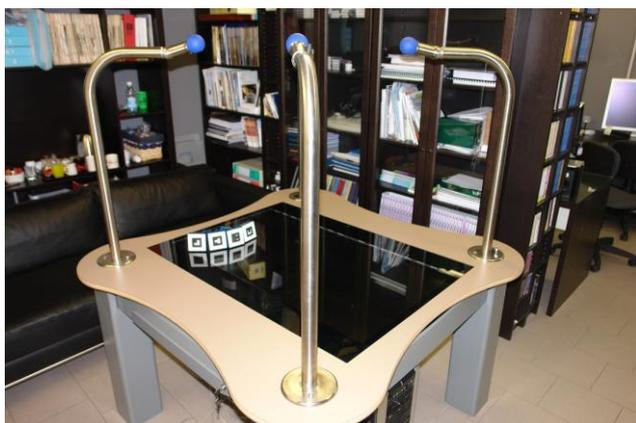
**Fig. 1.** The Eldergames prototype with the 4 pens on the table top and the cameras lodged in the 4 blue spheres.
