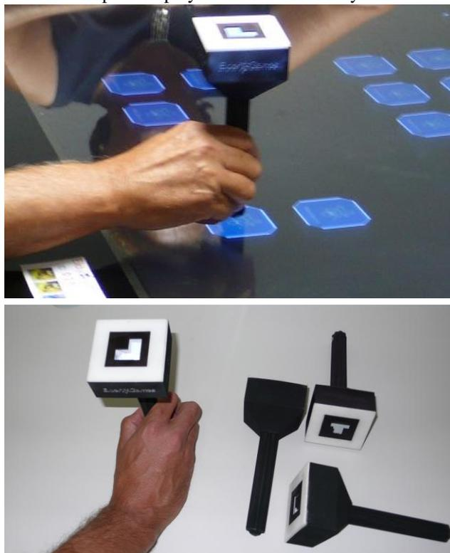
**Fig. 2.** The objects/pens used to interact with the table.
